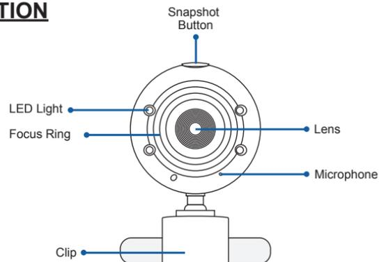
**NOTE:** To adjust focus use the Focus Ring located in front of lens.
