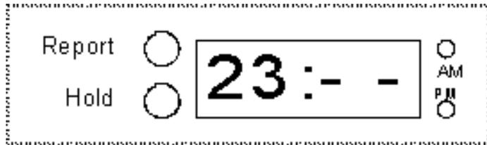
Press **select** a sixth time (note the colon between the hours and minutes), and the unit will display minutes. Press the **maximum** or **minimum** buttons.
