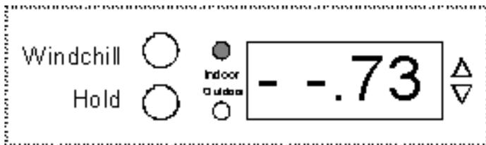
Press **select** a third time - the unit displays the outdoor temperature. Press the **maximum** or **minimum** key to enter the actual temperature.
