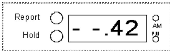
Press **select** a seventh time (note only the right two digits); the unit will display seconds. Press the **maximum** or **minimum** buttons to set the seconds. (note: the seconds is updated on the display only when the maximum or minimum button is being depressed).
