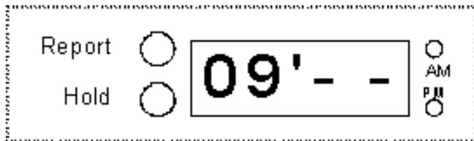
Press **select** an eleventh time (the single dot remains at the top between the hour and minute), and the minutes of the peak hour will be displayed. Change as desired.
