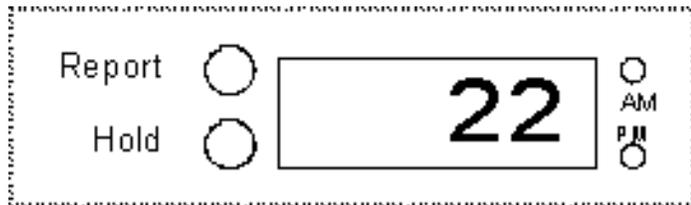
Press **select** a eighth time (a single dot at the bottom separates the hour and minute); the lunar/tide clock will display the number of hours in a cycle.
