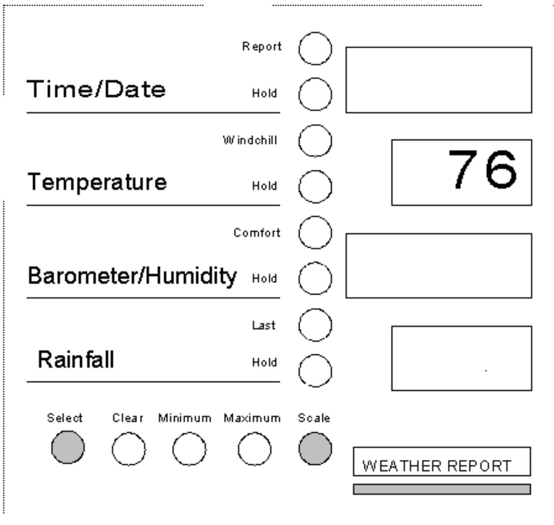
Press **select** a second time and the unit displays the indoor temperature. Press the **maximum** or **minimum** key to enter the actual temperature.
