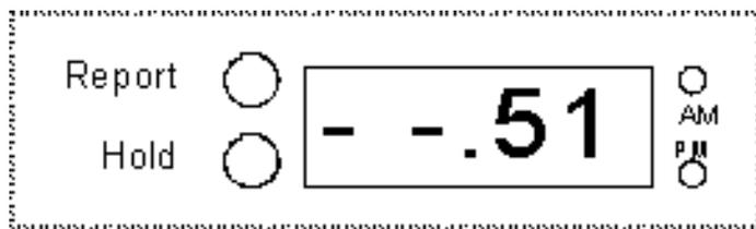
Press **select** a tenth time (the single dot is now located at the top, between the hour and minute); the peak of the cycle hour (usually high tide) will be displayed. Change as desired.
