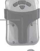
To use the belt clip as a stand, remove the belt clip from the back of the monitor. Insert the left or right side of the clip into the lower part of the slot. Then snap the other side of the clip into the other lower slot.
