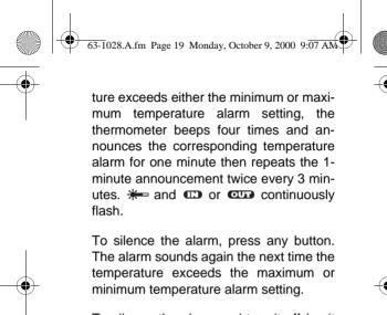
To silence the alarm and turn it off (so it does not sound again), press ALARM ON/
