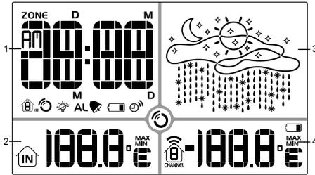
1. **Clock / Alarm / Calendar Area:** Radio-controlled clock; alarm; calendar
