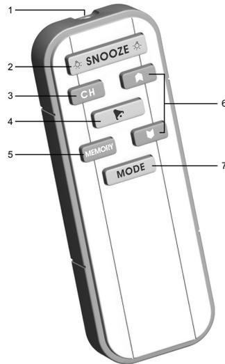
1. Infrared signal transmitter
