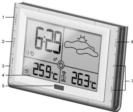
1. **CHANNEL:** Switch remote sensor display
