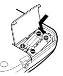
**3** Connect the AC power adaptor. The indication "CHG" lights up. Charge for about 2 hours (for BP-DM10) or 3.5 hours (for BP-DM20). (If the battery has been fully charged,
