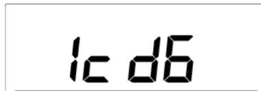
**Note:** There are 8 LCD contrast levels to choose from—“Lcd 0” is the lightest, and “Lcd 7” is the darkest.
