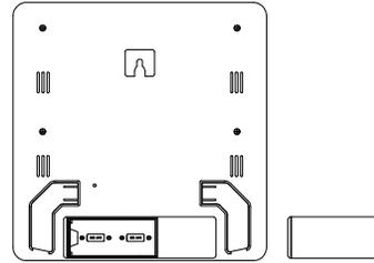
1. Insert finger or other solid object in the space at the bottom center of the battery compartment and lift up to remove the cover.
