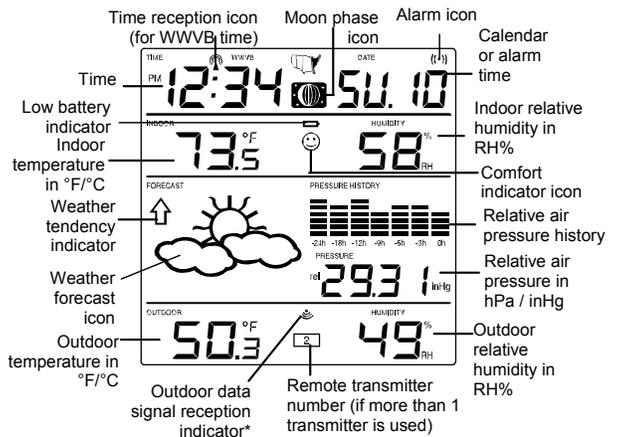
\* When the signal is successfully received by the Weather Station, the outdoor transmission icon ☀ will be switched on. If not successful, the icon will not be shown on LCD. The user can then easily see whether the last reception was successful (icon on) or not (icon off). A short blinking of the icon indicates that signal reception is currently taking place.
