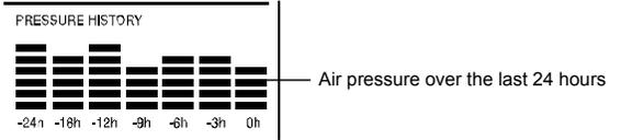
The bar chart indicates the air pressure history trend over the last 24 hours in 7 steps, 0h, -3h, -6h, -9h, -12h, -18h, and -24h. The "0h" represents the current full hour air pressure recording. The columns represent the "hPa" (0, ±2, ±4, ±6) at specific time. The "0" in the middle of this scale is equal to the current pressure and each change (±2, ±4, ±6) represents how high or low in "hPa" the past pressure was compared to the current pressure.
