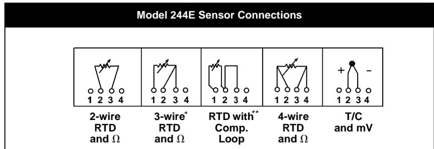
\* Rosemount Inc. provides 4-wire sensors for all single element RTDs. You can use these RTDs in 3-wire configurations by leaving the unneeded leads disconnected and insulated with electrical tape.
