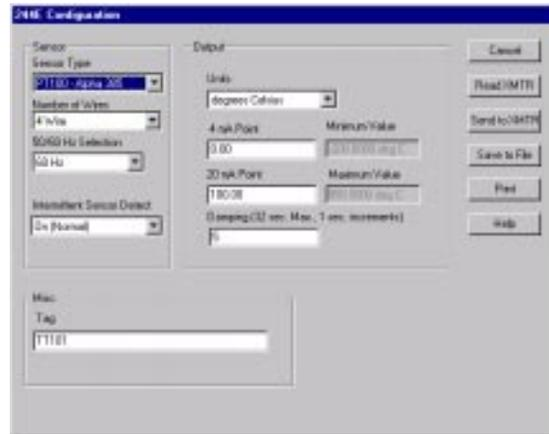
4. Set the configuration parameters. To view a complete list of options for each parameter, click the drop-down arrow in any parameter box. For example, on the main configuration screen, click the arrow in the **UNITS** box to view a list of available units.
