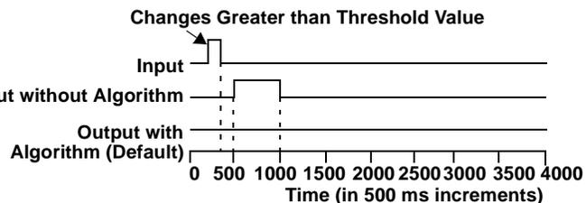
C) If any of the next three measurements is outside the new threshold value (at Time = 500 ms), the output remains unchanged at the initial reading (Time = 0 ms). the transmitter remains in a hold period until four consecutive measurements are within the threshold value of the first in the series.
