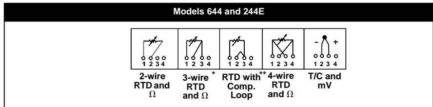
\* Rosemount Inc. provides 4-wire sensors for all single element RTDs. You can use these RTDs in 3-wire configurations by leaving the unneeded leads disconnected and insulated with electrical tape.
