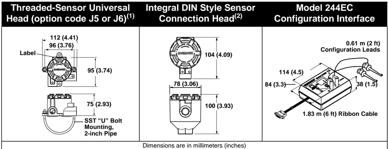
(1) A "U" Bolt is shipped with each universal head unless assembly option code X1, X2, or X3 is ordered. However, since the head can be integrally mounted to the sensor, it may not need to be used.
