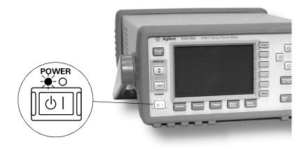
3. Turn the meter on and confirm the green LED is lit.
