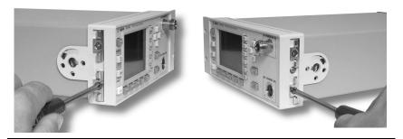
6. Engage the linking plates at the front of the power meters.
