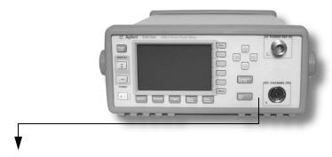
These keys and connectors are associated with the measurement channels and are located on the right-hand side of the front panel.
