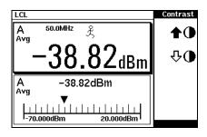
Diagram shows display with an E-series E9320 power sensor connected. 5. Connect the sensor to the POWER REF connector.
