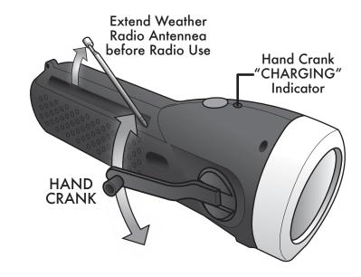
The Hand Crank charges the included pre-installed 3.6v Ni-MH battery pack which will power one of the following functions for a specified amount of time:
