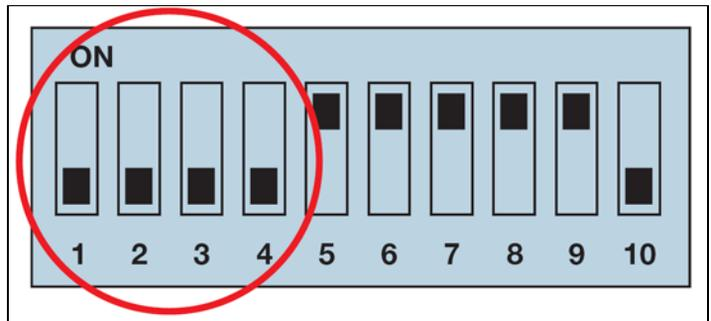
Also on the S3 mini-dip switch, verify that position 10 selects the correct video format—NTSC or PAL. The following diagram shows the switch in the NTSC setting.
