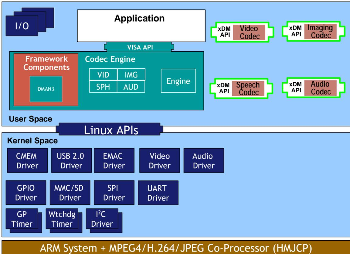
In the previous figure, everything runs on the ARM. The application handles I/O and application processing. To process video, image, speech, and audio signals, it uses the VISA APIs provided by the Codec Engine. The Codec Engine, in turn, uses xDM-based codecs. For more information, see the *Codec Engine Application Developer's Guide* (SPRUE67).
