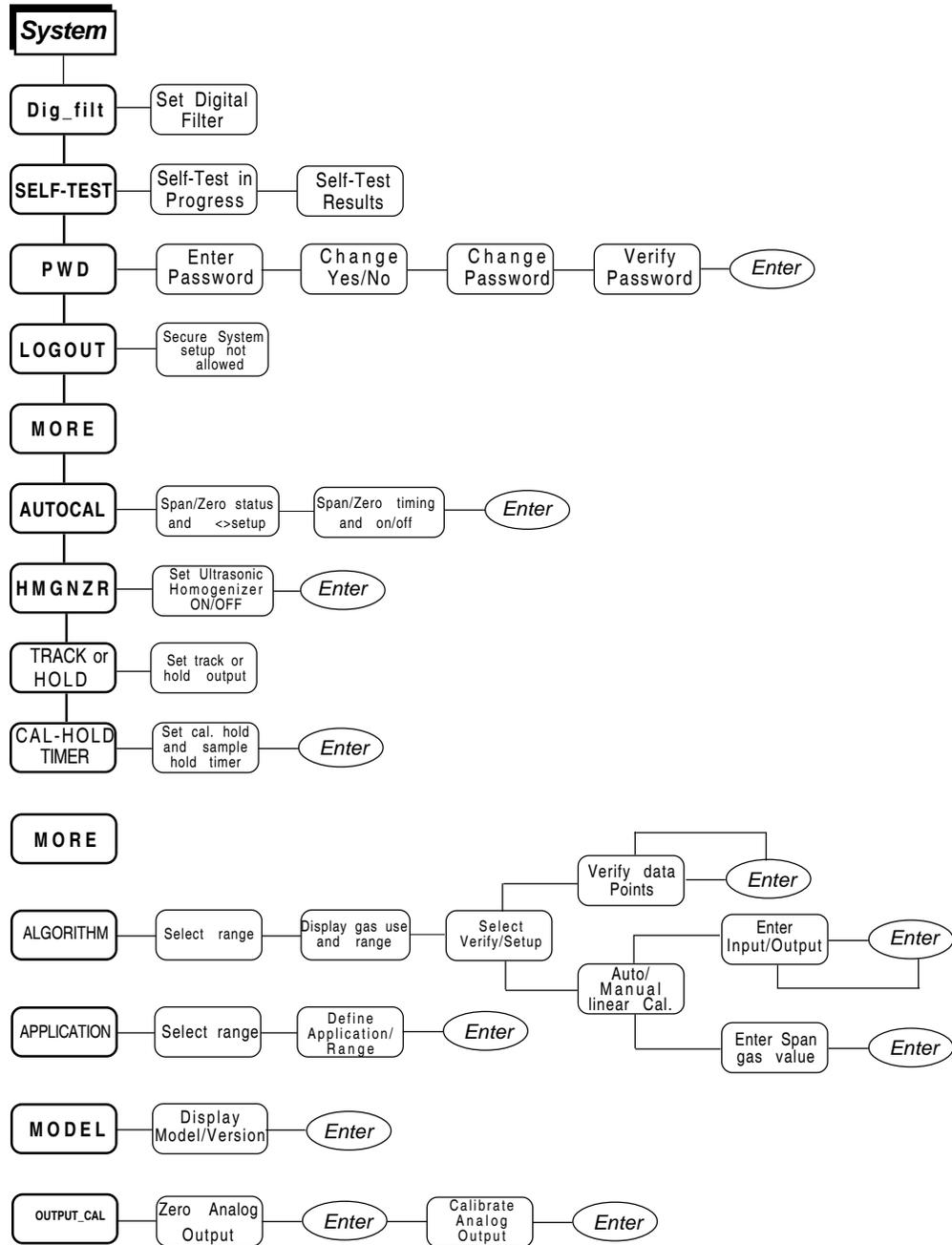
Figure 3-1: Hierarchy of System Functions and Subfunctions
