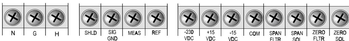
The first strip terminal has three contacts labeled N, G and H. The labels stand for Neutral, Ground, and Hot. This is the AC power strip terminal. It feeds AC power to other components of the Model 6600 System, such as the D2 lamp power supply, heater, and temperature controller PCB.
