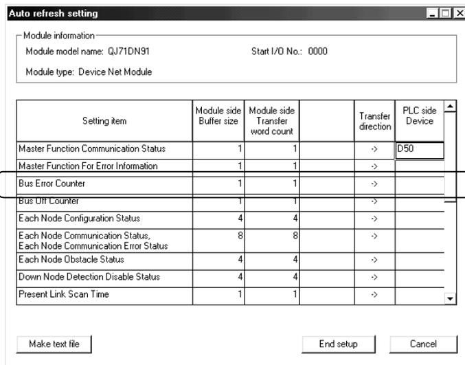
The number of settings in this one line is counted as one setting. The number of settings is not counted by columns. Add up all the setting items in this setting screen, then add them to the total for the other intelligent function modules to get a grand total.
