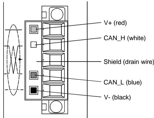
The figure above shows the QJ71DN91's DeviceNet connectors. A sticker in the corresponding cable color is pasted on each connector.
