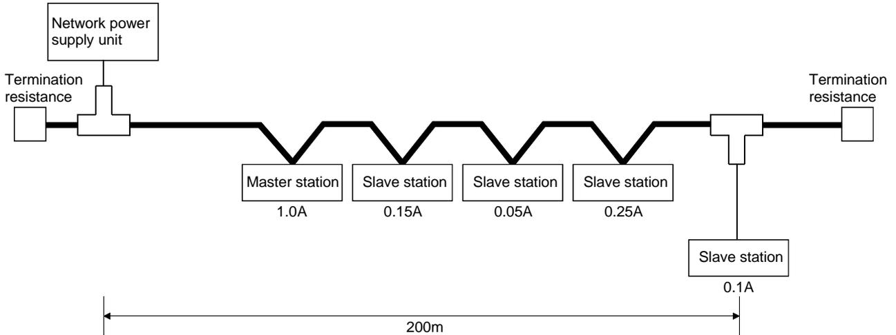
Thick-cable power supply distance = 200 m
