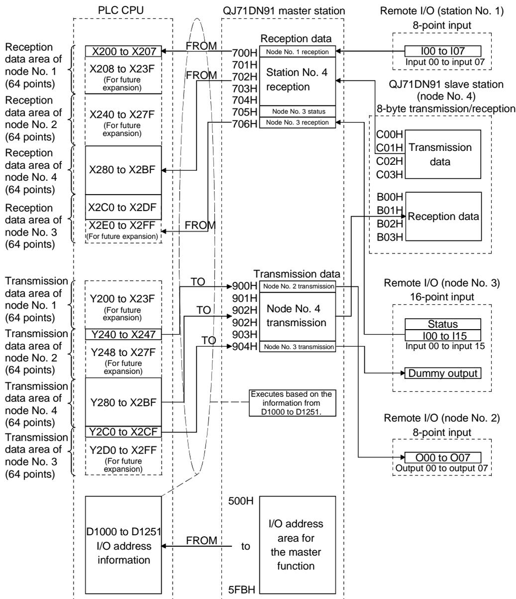
The following explains an example of the sequence program used in this case.
