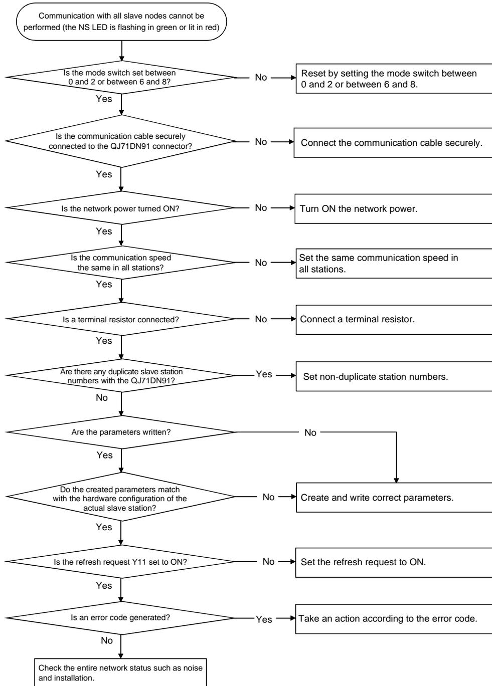
9.1.3 When communication with a specific slave node cannot be performed (using the master function)
