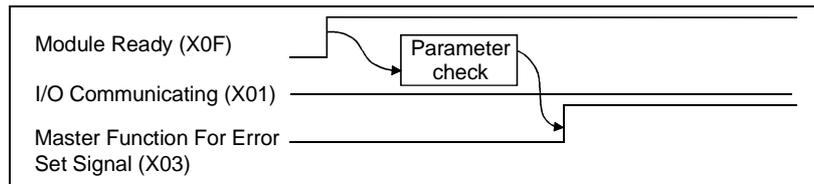
(3) I/O Communicating : X01, I/O Communication Request: Y11 (when the slave function is used)
