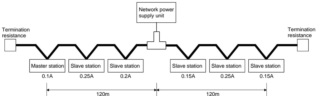
Power supply distance left of the network power supply unit = power supply distance right of the network power supply unit = 120 m
