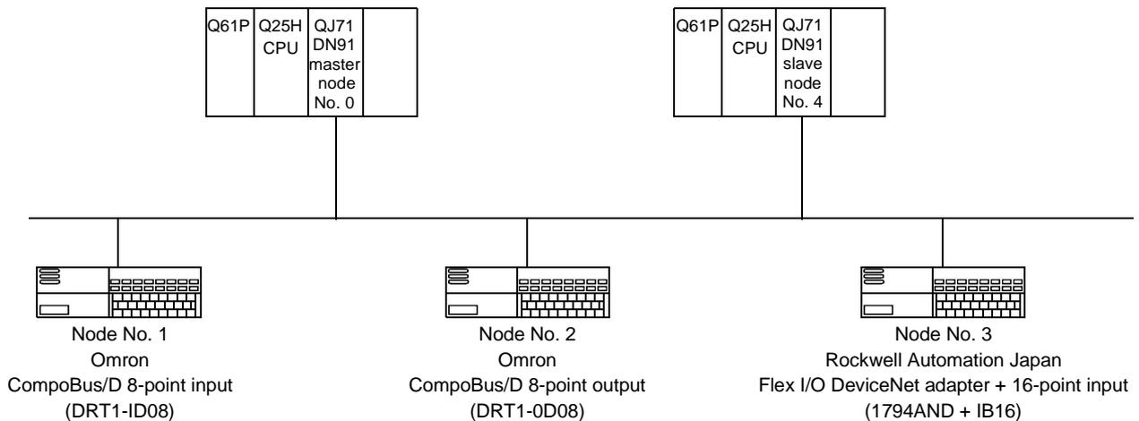
\* The Flex I/O DeviceNet adapter by Rockwell Automation Japan has 2-byte input data as a status, as well as 2-byte input data and 2-byte output data.
