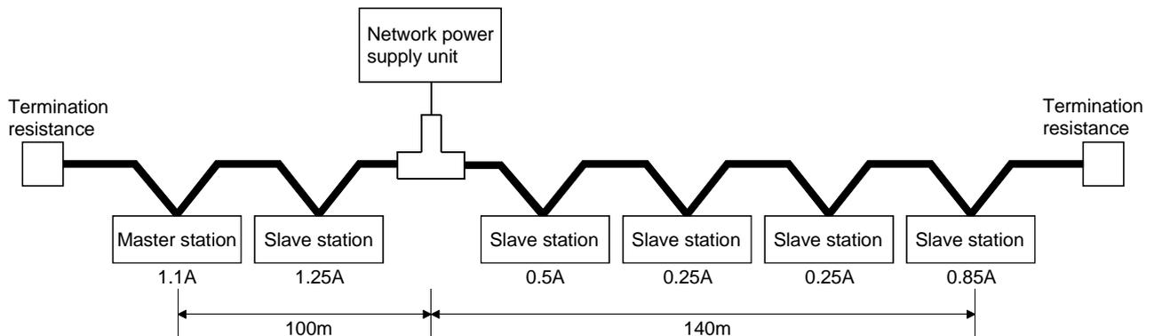
Total power supply distance left of the network power supply unit = 100 m
