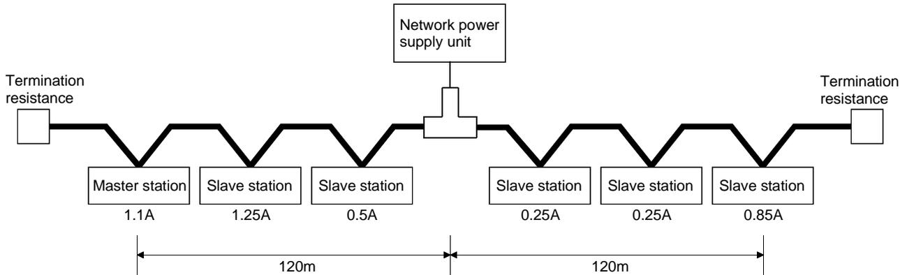
Power supply distance left of the network power supply unit = power supply
