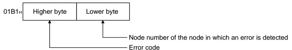
(1) When the error-detected node number (lower byte of error information) is FFH
