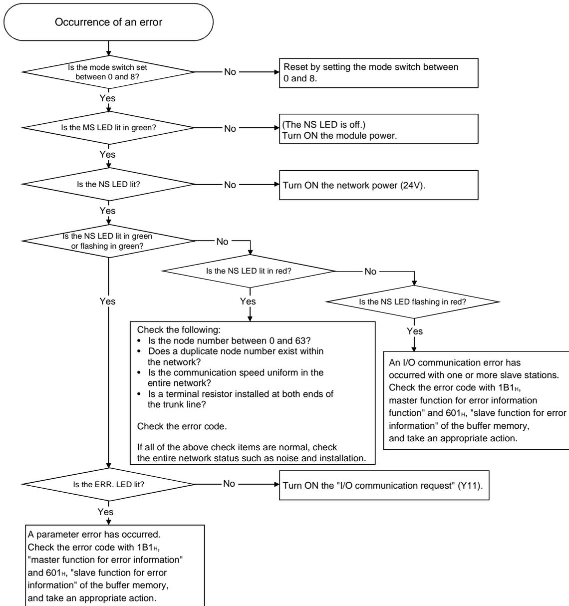
9.1.2 When communication with all slave nodes cannot be performed (using the master function)
