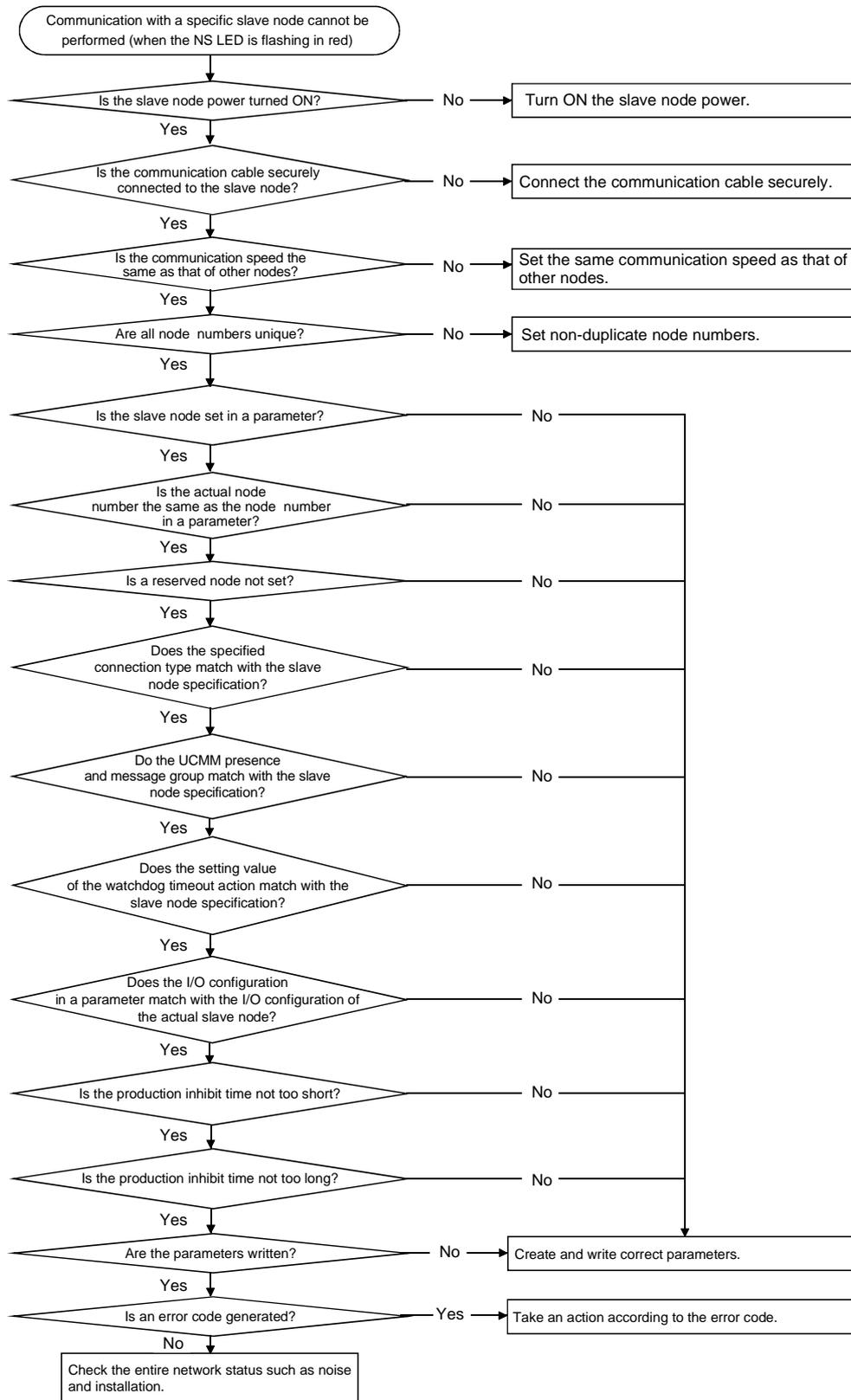
9.1.4 When communication with the master node cannot be performed (using the slave function)
