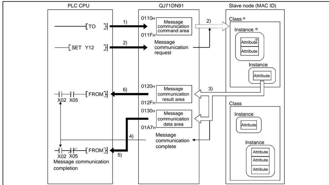
\*: In DeviceNet, the area used for reading and writing via communication is specified by the numbers representing the class ID, instance ID, and attribute ID. For details, refer to the manual of each slave node.
