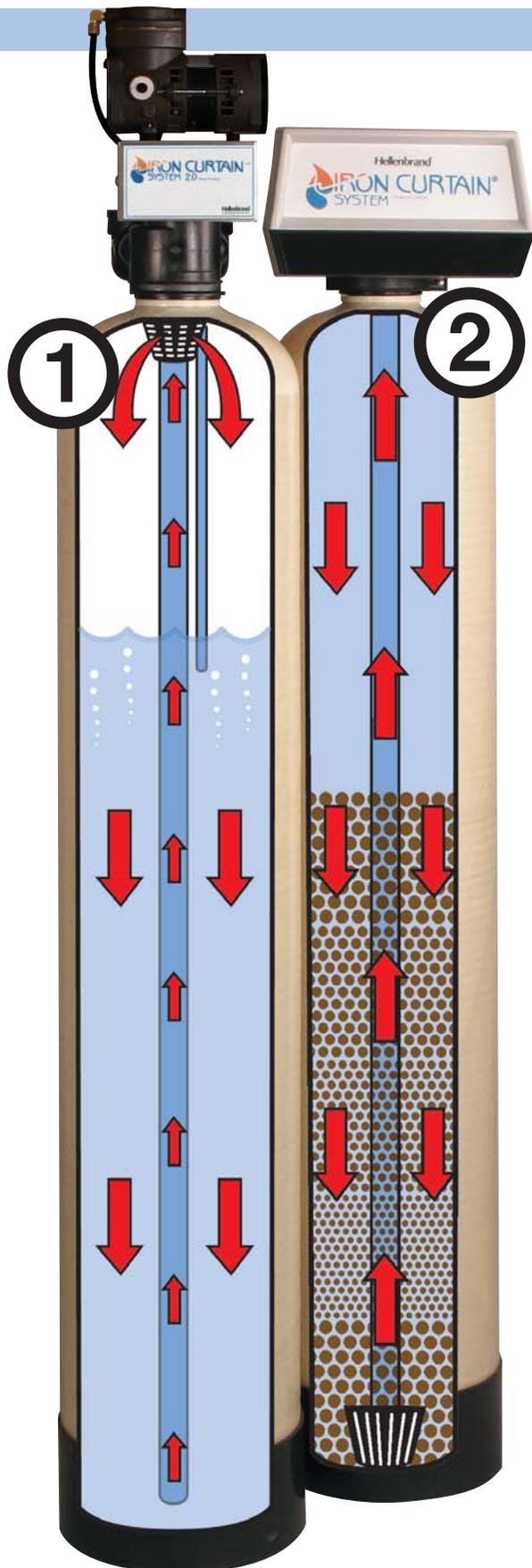
The Iron Curtain™ Filtration System is among the simplest, most economical and effective iron filters available. It removes iron, sulfur, and manganese from water.
