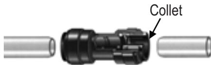
Cut the tube square. It is essential that the outside diameter be free of score marks and that burrs and sharp edges be removed before inserting into fitting.
