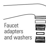
**NOTE:** Adapters and gaskets have been included to connect to most faucets. To insure a leak-free seal, you may need to use your existing gasket (removed during Step 1) from your faucet's aerator in addition to the gasket included with this system. If the adapters will not connect to your faucet, it is recommended to consult a local plumbing or hardware store for assistance in obtaining the correct adapter for your faucet.
