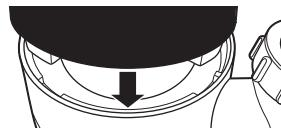
**NOTE:** The cap is designed to fit on the filter housing only one way.
