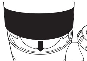
**NOTE:** The cap is designed to fit on the filter housing only one way.
