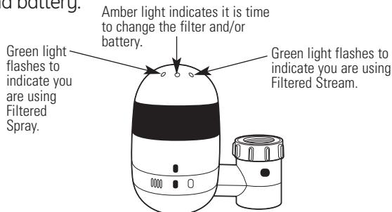
The amber light will flash one time every few seconds to remind you that it is time to change the filter. The amber light will flash three quick flashes every few seconds when it is time to change the battery and filter.
