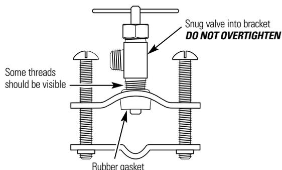
*Optional water supply connection (using saddle valve)\**
