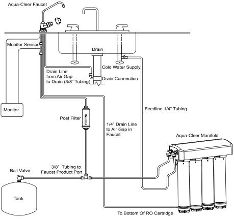
**Note:** Install the drain line so that it runs downward with no loops or low spots. Otherwise the unit will overflow at the air gap siphon break built into the faucet, or make irritating gurgling sounds. The 1/4" concentrate line that leads to the faucet should be installed in a straight vertical path to avoid making a gurgling noise.
