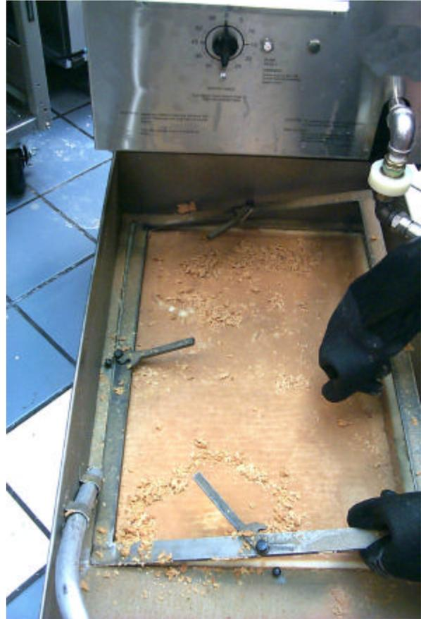
3. Roll both ends of the top filter paper into the center, making sure no sediment falls out, and discard. Remove the second sheet of filter paper and retain for re-use.
