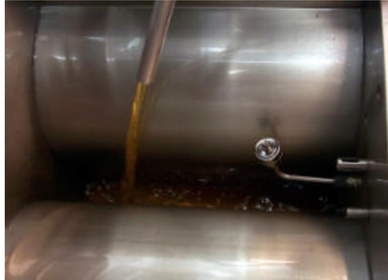
9. Close the drain valve handle. It takes approximately 5 to 7 minutes for the filter to pump all the oil back into the fryer.
