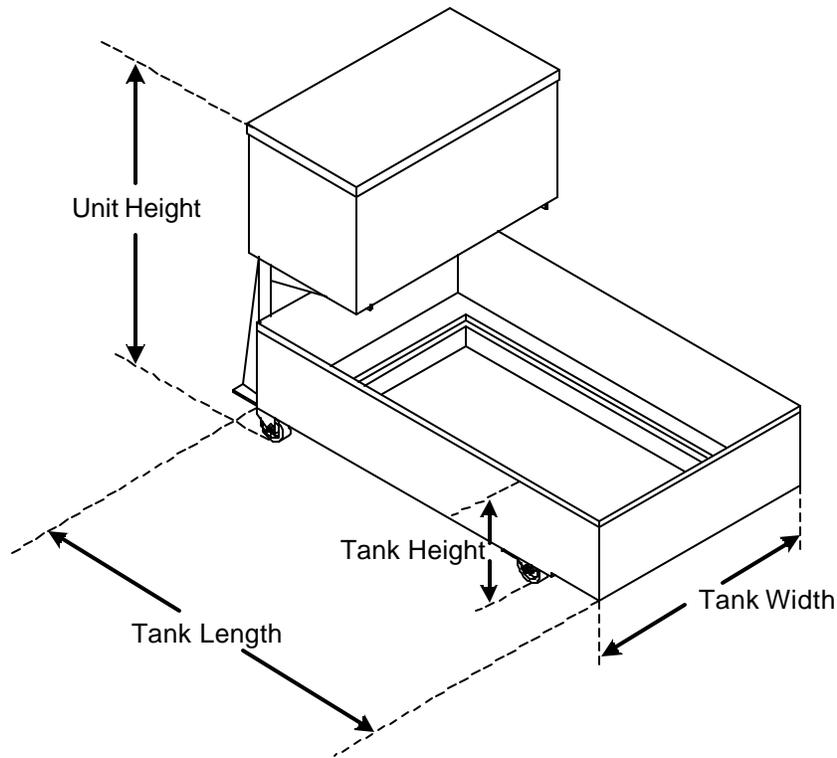
MF90 Series filter unit dimensions (unit and tank heights are measured from bottom of casters to top of unit and tank, respectively).
