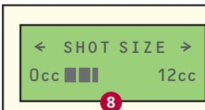
\*Speedbar™—This feature is available in the volume input, dispense rate input and backoff input. Hold down the left or right arrow key to make this feature appear. Continue holding to make the bar increase or decrease. The longer you hold, the faster the bar moves. When satisfied, release the key and Speedbar™ will show you your selected volume.
