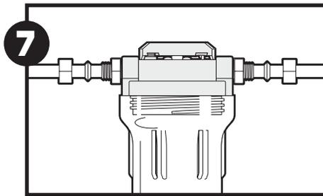
8. Turn on main water supply. Slowly turn handle on housing 1/4-turn counterclockwise to allow system to fill with water. Press red pressure-relief button on top of filter to release trapped air. Check for leaks, then rotate handle fully to "ON" position. Open nearest faucet and flush filter cartridge for 15 minutes.
