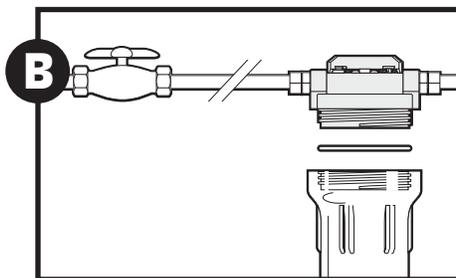
C. Screw the bottom of housing onto the cap until it is hand-tight. Do not over-tighten. Slowly turn handle on housing 1/4-turn counterclockwise to allow system to fill with water.
