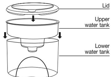
3. Carefully lift the flip top lid and add **cold** water to the **FILL** line. **NOTE:** This is a gravity fill system. To increase the filtering flow rate, continue adding water to the **FILL** line of the upper tank until tanks are completely full.
