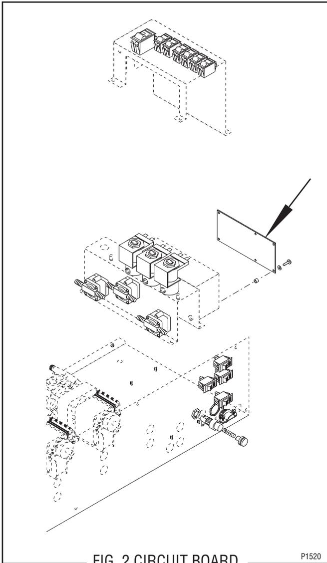
FIG. 2 CIRCUIT BOARD
