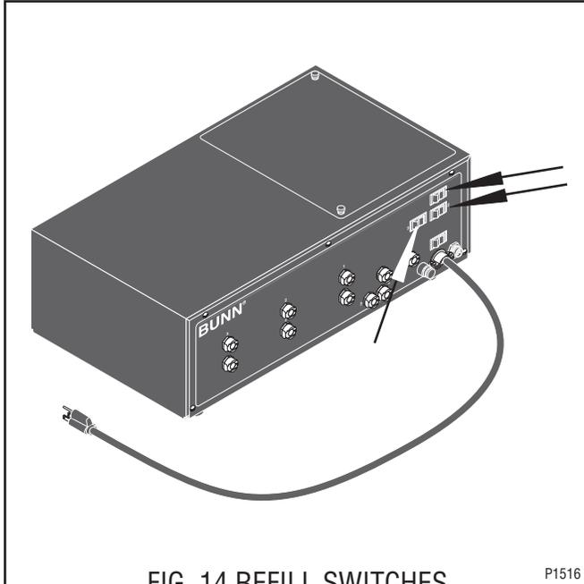
FIG. 14 REFILL SWITCHES
