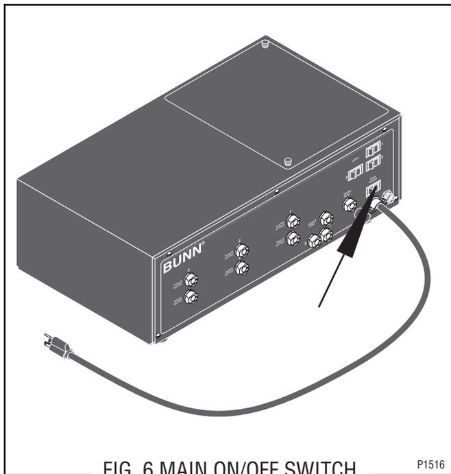
5. Check for continuity across the switch terminals with the switch in the "ON" position. Continuity must not be present when the switch is in the "OFF" position.
