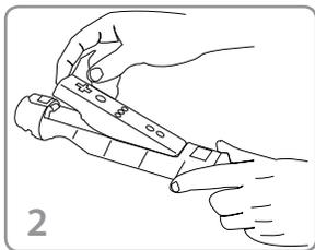
■ **Insert the bottom of the Wii remote into base of the handle.**
