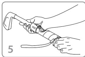
**To attach any sports attachment align the release button on the back of the sport handle with the base of the sports attachment and slide the attachment together until it snaps into place.**
