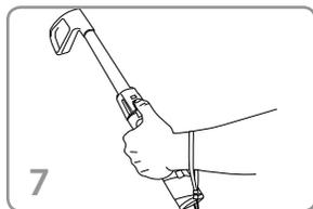
**To detach any sports attachment press the release button on the back of the sport handle.**
