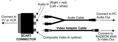
The above illustration shows how to connect your RADEON 8500 to a European TV using the SCART.
