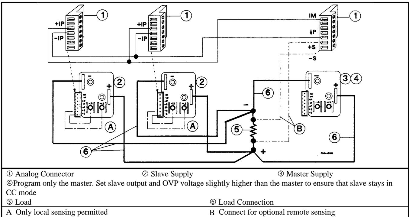
**Figure 4-4e. Series 667xA Auto-Parallel Connection (Remote Sensing Optional)**
