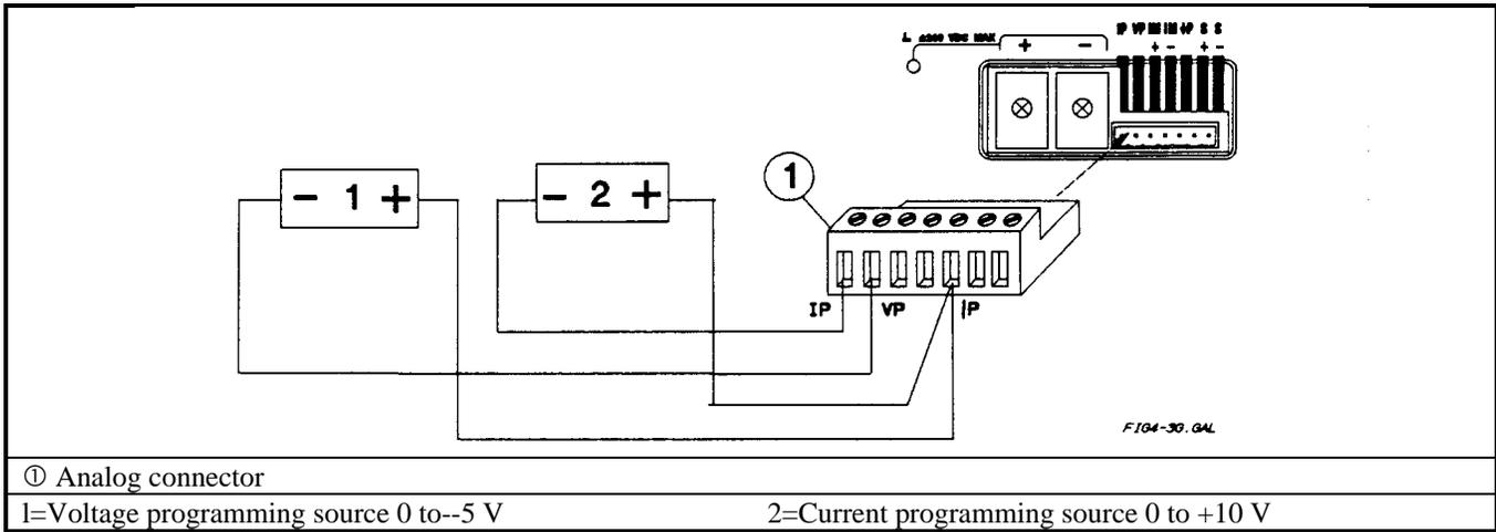
**Figure 4-3g. Series 664xA and 665xA Analog Programming Connections**
