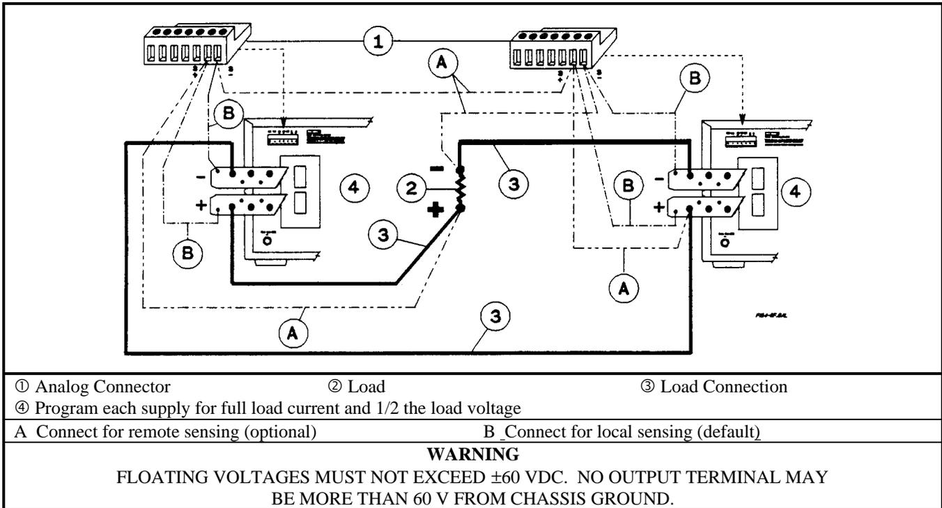
**Figure 4-5f. Series 668xA Series Connection (Remote Sensing Optional)**
