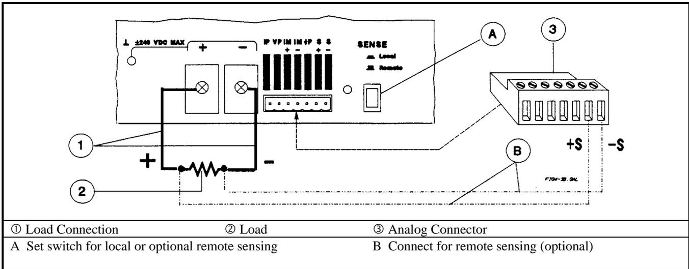
Figure 4-3b. Series 664xA and 665xA Single Load Connection
