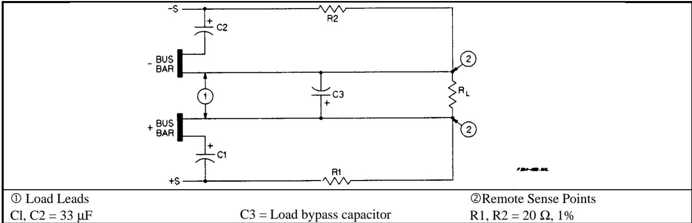
**Figure 4-4b. Series 667xA Sense Lead Bypass Network**
