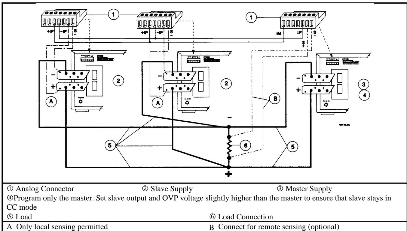
**Figure 4-5e. Series 668xA Auto-Parallel Connection (Remote Sensing Optional)**
