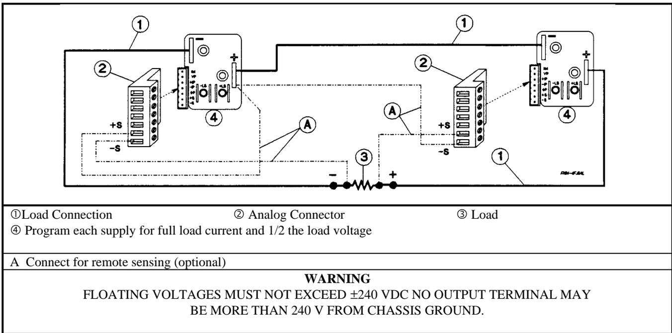
Figure 4-4f. Series 667xA Series Connection (Remote Sensing Optional)
