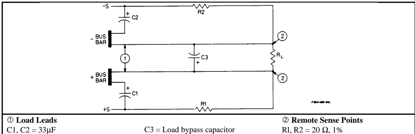
Figure 4-5b. Series 668xA Sense Lead Bypass Network
