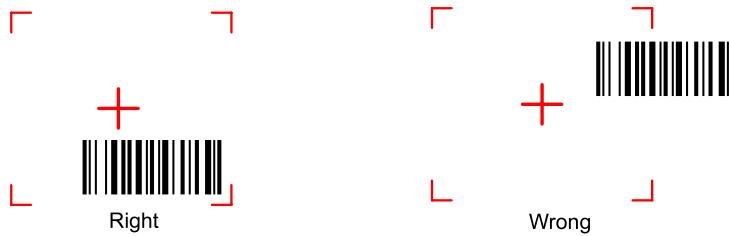
Figure 2-17 Bar Code Not Centered in Aiming Pattern
