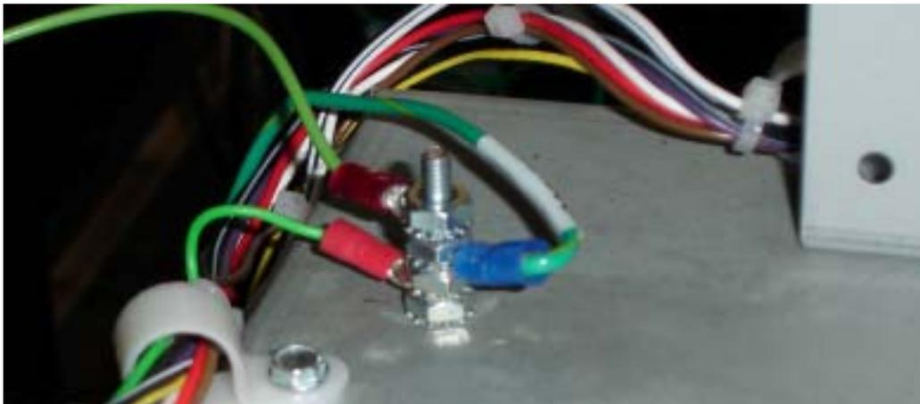
Figure 3. Coin Vault Ground Lug
