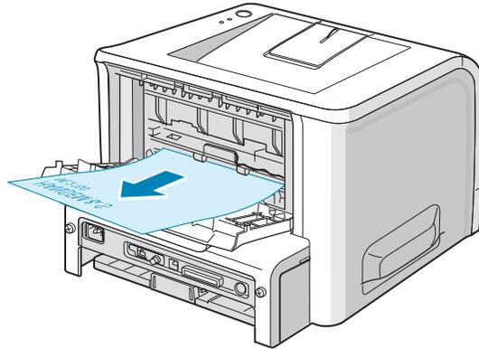
Printing from the Multi-Purpose Tray to the rear output tray provides a **straight paper path**. Opening the rear output tray might improve the output quality with the following:
