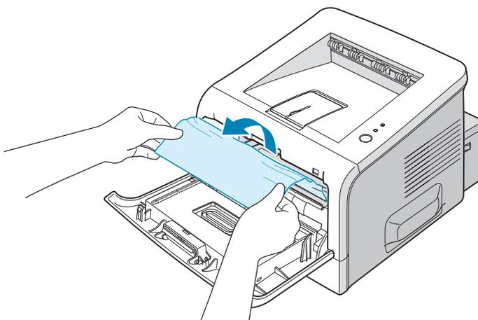
If the jammed paper is not visible or there is resistance when you pull the paper, go to "In the Paper Exit Area" on page 6.12.
