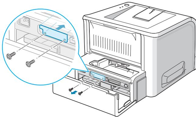
**5** Insert the front of the network interface card to the corresponding slot of the machine.
