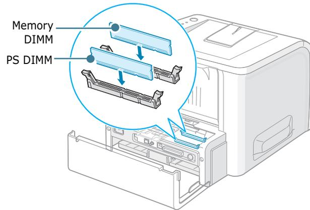
To install the memory DIMM, continue with Step 5.
