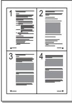
You can select the number of pages to print on a single sheet of paper. To print more than one page per sheet, the pages will appear decreased in size and arranged on the sheet. You can print up to 16 pages on one sheet.
