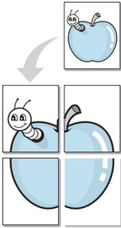
This feature allows you to print a single-page document onto 4, 9 or 16 sheets of paper, for the purpose of pasting the sheets together to form one poster-size document.
