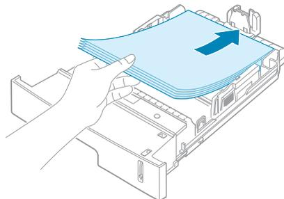
You can load previously printed paper. The printed side should be facing up with an uncurled edge on top. If you experience problems with paper feed, turn the paper around.
