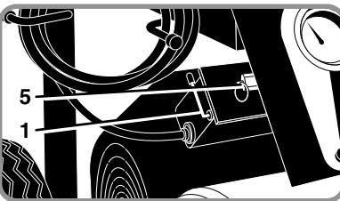
**2) MOTOR THERMAL OVERLOAD:** The electric motor has a thermal overload protector. If the motor overheats for any reason, the thermal overload will cut off power, thus preventing the motor from being damaged. Wait until the motor is cool. Motor has a circuit breaker. Reset switch if it is tripped.
