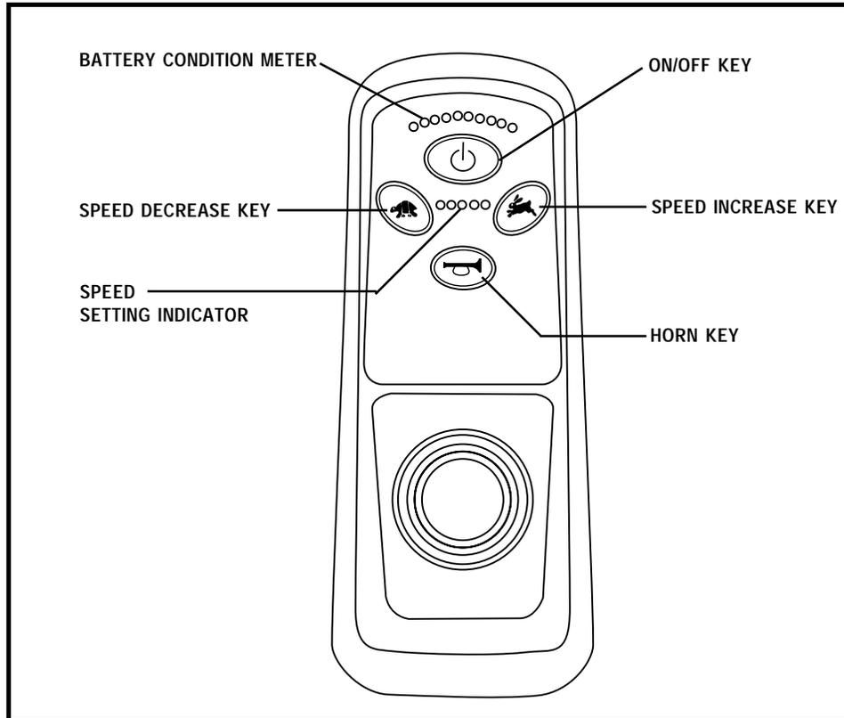
Figure 3. FLIGHT Keypad
