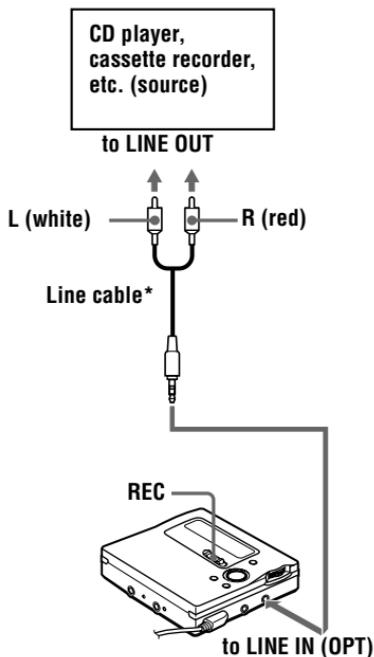
\* Use the connecting cords without an attenuator. To connect to a portable CD player having a stereo mini-jack, use the RK-G136 connecting cord. For more information on connecting cords, see "Optional accessories" (page 88).
