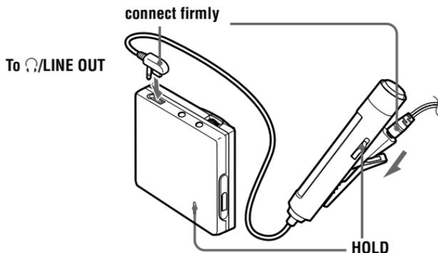
① Connect the headphones/earphones with the remote control to **LINE OUT**.
