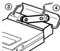
Insert a LR6 (size AA) alkaline dry battery.
