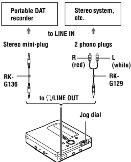
When connecting a line cable to the  $\odot$ /LINE OUT jack of the recorder, be sure to set the "AUDIO OUT" parameter for the  $\odot$ /LINE OUT jack.
