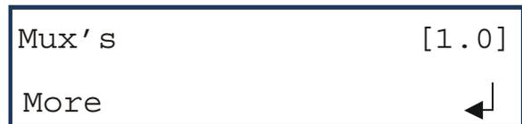
Using the figure, the LCD shows that the controller is at the Multiplexer Menu, which is menu 1. More indicates that there are more options or submenus available under this menu.
