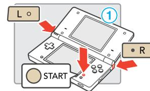
2. Press POWER. (Hold down the L, R, and START Buttons until the Calibration screen appears.)
