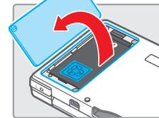
2. Remove the battery pack as shown at right.
