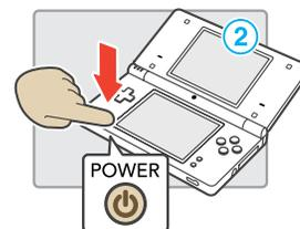
3. Follow the on-screen instructions and then turn the power off. Turn the system on again to check the operation of the Touch Screen.
