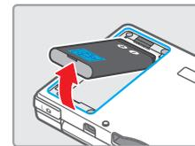
3. Orient the new battery as shown and carefully insert completely into the battery compartment.
