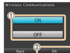
When the wireless communication function is turned on, the wireless light will flash.
