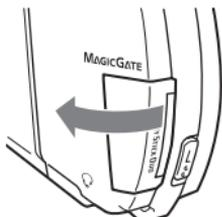
Open the slot cover in the direction of the arrow.
