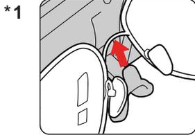
\*1 With certain eyeglass designs, the nose pad may catch the bridge of the eyeglasses and cause them to come out together with the display unit. To avoid this, remove the display unit as described above.
