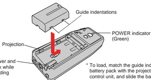
\* To unload, turn off the power and slide the battery pack back while pressing the battery unloading switch.
