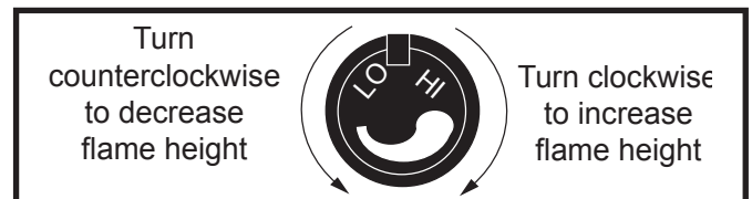
Fig. 42 Flame adjustment knob for Honeywell valve.
