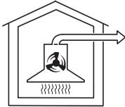
The hood comes equipped with a **non-return flap**. This flap automatically closes when the hood is turned off so that no exchange of outside air and room air can occur. When the hood is turned on, the air pressure of the exhaust fan automatically opens the flap blowing the inside air and cooking odors outside.
