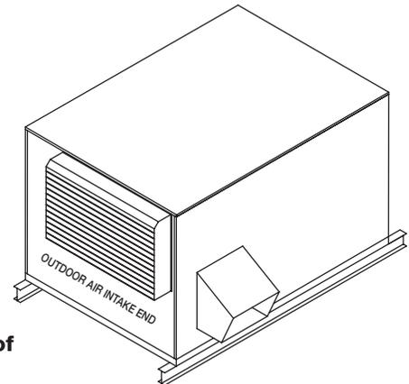
Isometric view of ERV on rails
