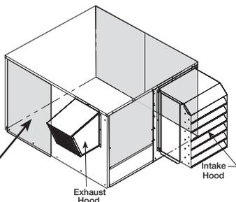
Access to Control Center Components is gained through the access panel indicated.
