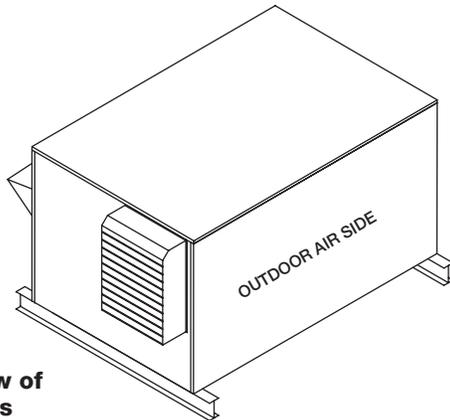
Isometric view of ERV on rails
