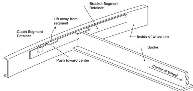
**Important!** Place retainers back in the original position before rotating the energy recovery wheel, otherwise damage to retainer will occur.
