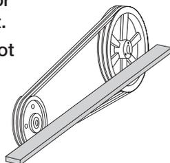
5. Place belts over sheaves. Do not pry or force belts, as this could result in damage to the cords in the belts.
