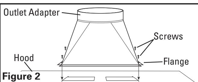
3. It is highly recommended that a back draft damper be installed to prevent outside air from flowing back into the home. Choose a back draft damper (available separately) sized to fit the diameter of the outlet adapter. Attach the back draft damper into the outlet adapter, press fit it into the round opening of the adapter until it is fully seated, making sure the damper opens away from the hood otherwise airflow will be restricted (Figure 3).
