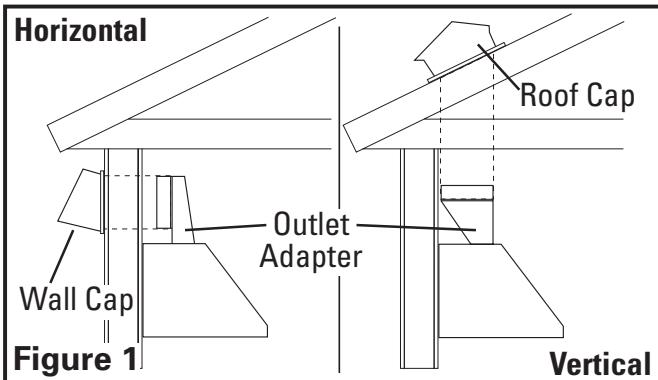
2. Install the proper sized outlet adapter (available separately) to the hood by matching up the four holes on the flange of the adapter to the four corresponding holes on the hood and secure in place with the provided screws. Ensure an airtight seal around the adapter by securing all connections with ducting tape (Figure 2).
