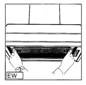
Remove old active carbon filters (always 2) by loosening the knurled screw in the centre.
