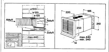
Abluft = Exhaust air Zuluft = Supply air
