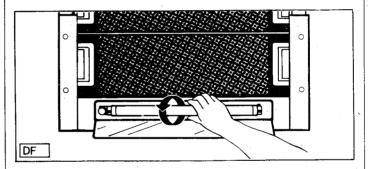
Important: Insert only a max. 15 W (860 D) or 16 W (8609 D) fluorescent lamp by twisting into the sockets to the right!
