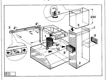
The wall rail can be horizontally aligned by shifting the sliding elements.
