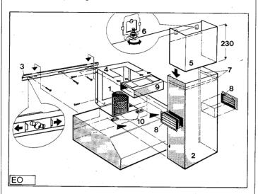
To connect the wall box/fume extractor hood, you are recommended to use the 125 mm dia. non-flammable exhaust air hose (E-No. 610899088) (for your own account from our range of special accessories). The exhaust air connection has a theoretical opening of 125 mm dia.
