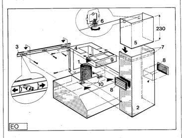
Preparing the wall box (exhaust air operation)
