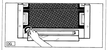
Insert a new starter by twisting to the right.
