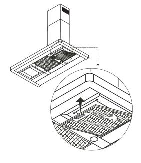
Metal Filter Dimensions: 16.12 in x 9.12 in 409 mm x 232 mm
