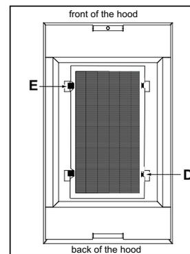
Install charcoal filter (plastic side exposed) into charcoal filter bracket. Insert tab cut-out side D of charcoal filter into bracket first. Lock charcoal filter into place by pushing down on side E with locking tabs.
