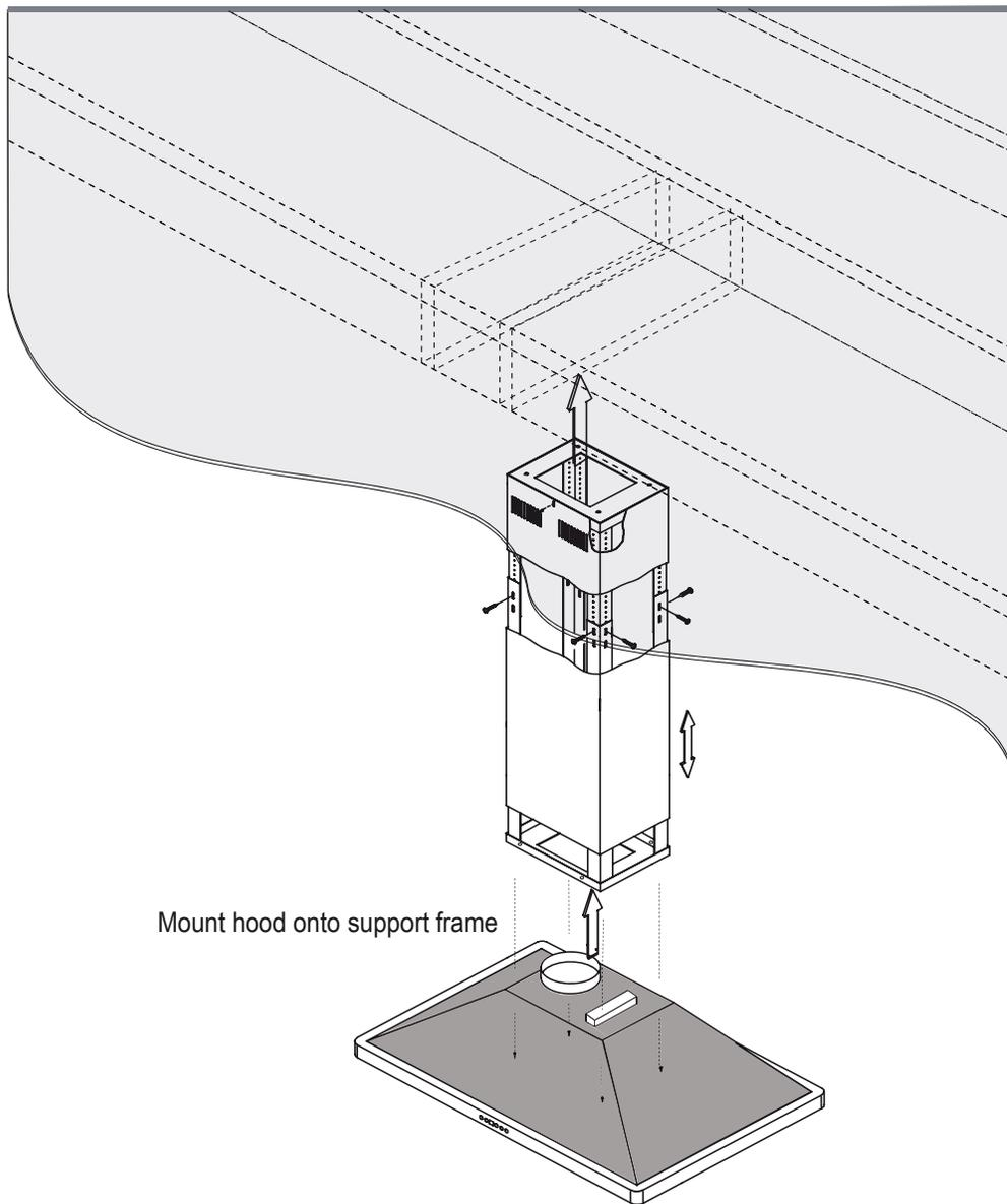
6. Lift lower duct cover and hood body onto bottom of support frame.
