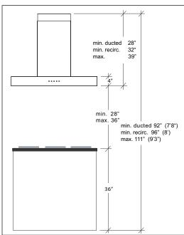
Note: Bottom duct covers may be cut down by 4" to expose top duct cover louver holes. This may be necessary if the customer is recirculating the hood, has an 8' ceiling and wants the hood mounted between 29 - 32 inches above the cooking surface.
