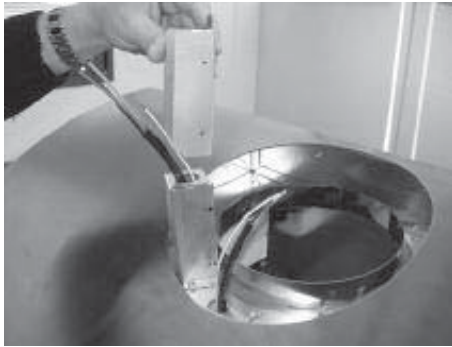
6. Position cover onto external blower wiring box.
