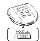
Slide HOLD in the direction of the arrow. When you press any button, "Hold " appears in the display and you cannot operate the player
