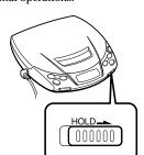
Slide HOLD in the direction of the arrow. When you press any button, "Hal d" appears in the display and you cannot operate the
