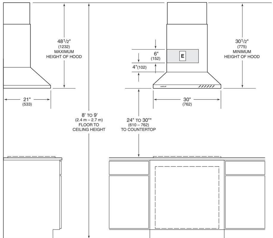
\*8' (2.4 m) ceilings will not allow for a 30" (762) maximum height above the countertop. Based on a 36" (914) high countertop, an 8' (2.4 m) ceiling will allow for a maximum height above the countertop of 29<sup>1</sup>/<sub>2</sub>" (749).
