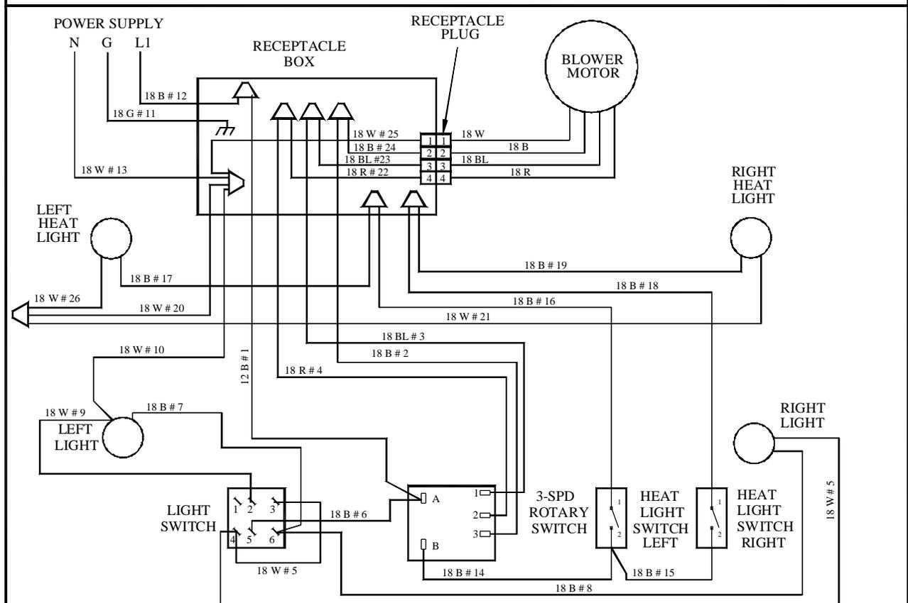
WIRING DIAGRAM-INTERNAL BLOWER, LIGHTING & HEAT LAMPS
